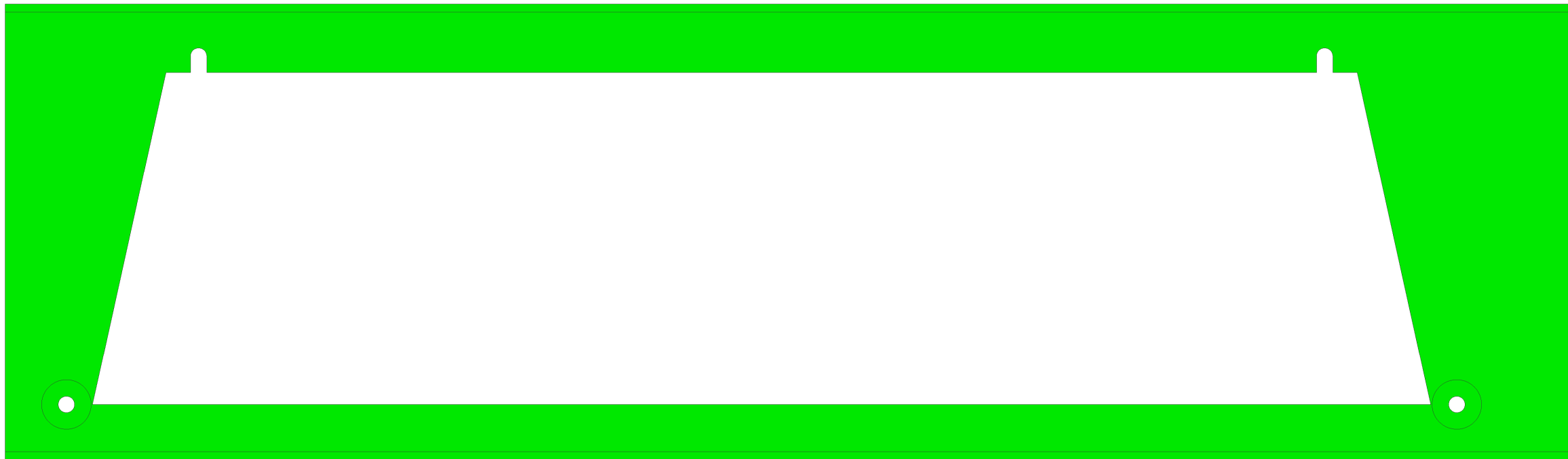
Battery Box Side Hole Xtd - Make 1 .1875 thick. Edge & Magnet pockets are .125 deep
