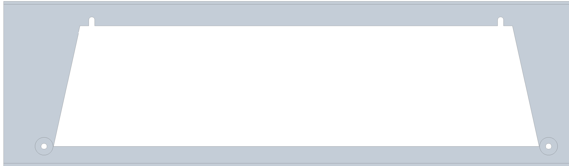
Battery Box Side Hole Xtd Mirror - Make 1 .1875 thick. Edge & Magnet pockets are .125 deep
